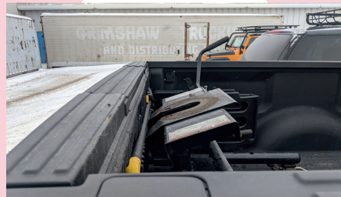
Fifth wheel hitch can be moved further back.
